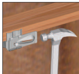
6: Tap Single Walers with hammer to tighten. Place 2x4 strongbacks (if desired) and secure with Form Aligner Clamps.
